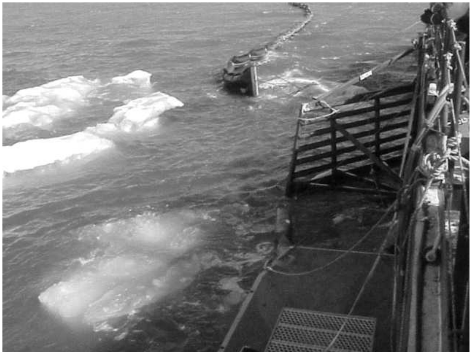
Figure 3-13: Example of ice deflection grate (Photograph by K. Ballard, ADEC 2000)
