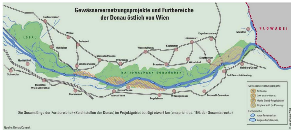
Figure 4.4: Water network projects and ford areas of the Danube east of Vienna. The total length of fords (shallow stretches) in the project area is about 6 km (ca. 15% of total length). (Source: DonauConsult)
