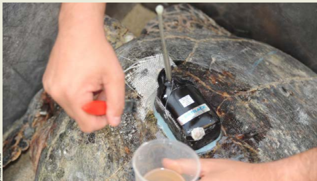
Figure 6: PTT being affixed on top of the turtle carapace using fibreglass cloth and resin.
