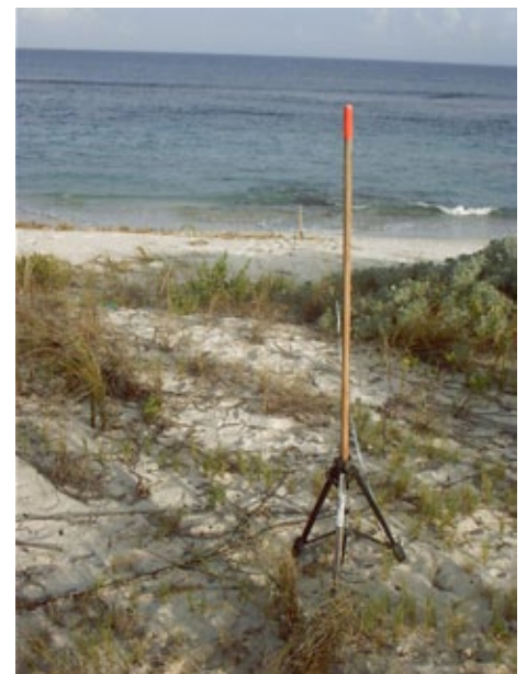
Figure 2. Using a tripod and pole to measure a beach profile.
